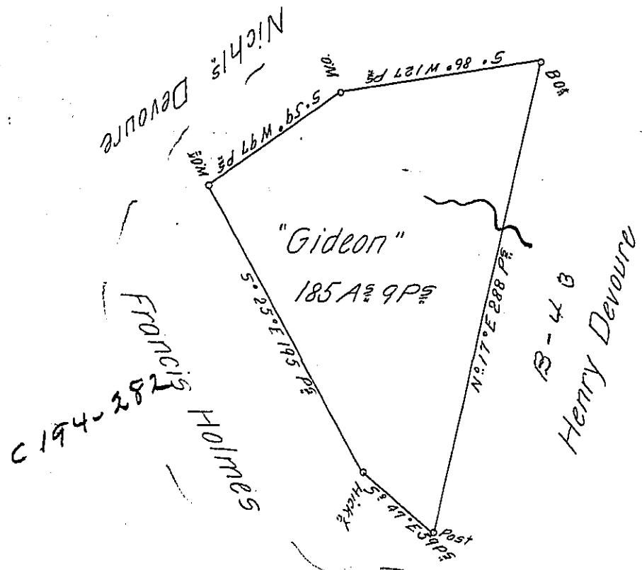
A Draught of a Survey called "Gideon" situate on the Waters of Mingo Creek in Washington County containing 185 A<sup>s</sup> 9 P<sup>s</sup> and the usual Allow<sup>ee</sup> for Roads &c executed Apr<sup>t</sup> 1<sup>st</sup> 1788 in Pursuance of a Warrant granted to Henry Devour for 200 A<sup>s</sup> dated Feb<sup>r</sup> 21<sup>st</sup> 1788.
